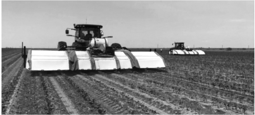
John Deere has acquired Blue River Technology, maker of 'smart' machines like the See & Spray, which uses artificial intelligence to identify weeds and robotic sprayers to dose them with herbicide. (Blue River Technology)
