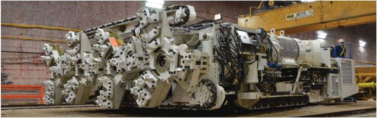
Mosaic's ninth four-rotor miner left Mosaic's new four-rotor assembly shop recently, clearing the way for the tenth miner that is scheduled to be assembled and in production by October.
