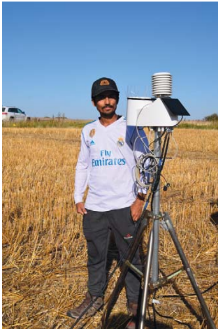
Bhuwan Bhandari leads the cover crop trial utilizing soil moisture sensors analyzing soil salinity, moisture and leaf wetness comparing cover crops to non cropped areas.
