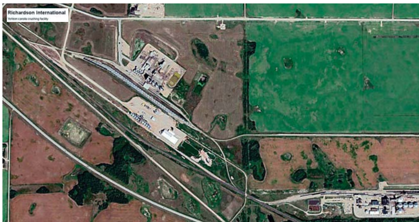
This Google Earth image shows the Richardson International canola crush facility at Yorkton on the left side of the map. To the right is the area where the triple loop track will be installed. The rail line going northwest/southeast is the Canadian Pacific mainline. The line going straight east connects to the CN rail network. The facility on the lower right is the Louis Dreyfus Company canola crush plant.
